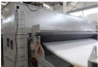
The Pre needling bonds the fiber at the initial stage, giving the fabric some structure. This needling process is fitted with the top needle boards, with density of 2500-3000 needles and the initial level of bonding between the different layers of felt happens at this stage.
