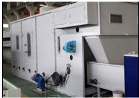
The machine is used to mix fully and store the pre-opened fiber for next working procedure, to ensure smooth production. The blender has a capacity to store almost 1 tonne of material in open form, this helps in saving the downtime whilst there is a change in the production quality, it also acts as a homogenous blender, wherein it blends the fibres perfectly in cases where two different types of fibres are used.
