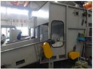
In this, fibres are manually fed and fiber mix percentage is decided, after which all the other processes take place continuously. The bale opener is equipped with the load sensors which directly control infeed to the line. The bale opener is specifically designed to process the fibres used in geotextile manufacturing and have a capability to process various types of fibres.
