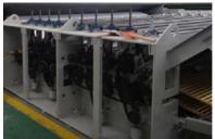
This web draft is part of a nonwoven production line and is between the lapper and needle to draft the multilayers of web and reach required specification. The drafting arrangement helps in uniforming the fabric properties across and along the width of the fabric (machine direction and cross direction). This helps in achieving more uniform fabric properties.
